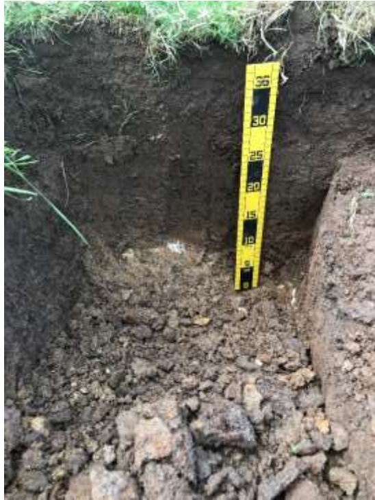
2. HC4 Ditch with clay soil
