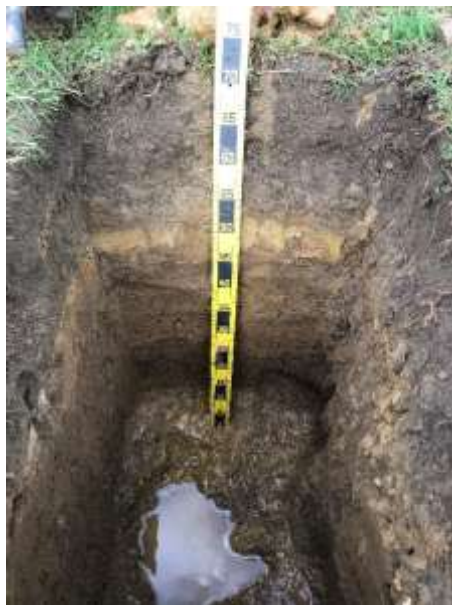
8. HC10 Section with clay layer at 200 mm
